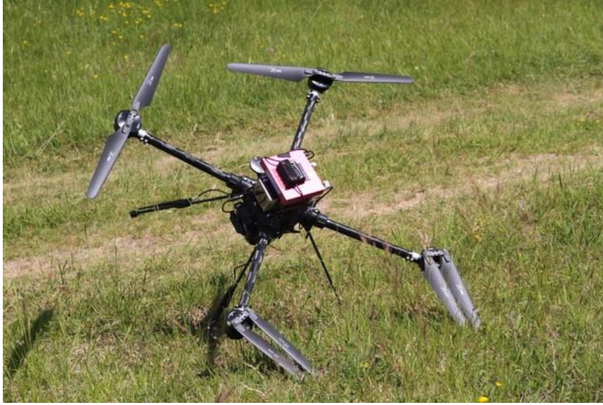
Figure 13: the "rapace" was not able to take off, because its algorithms misjudged the nature of the grass
