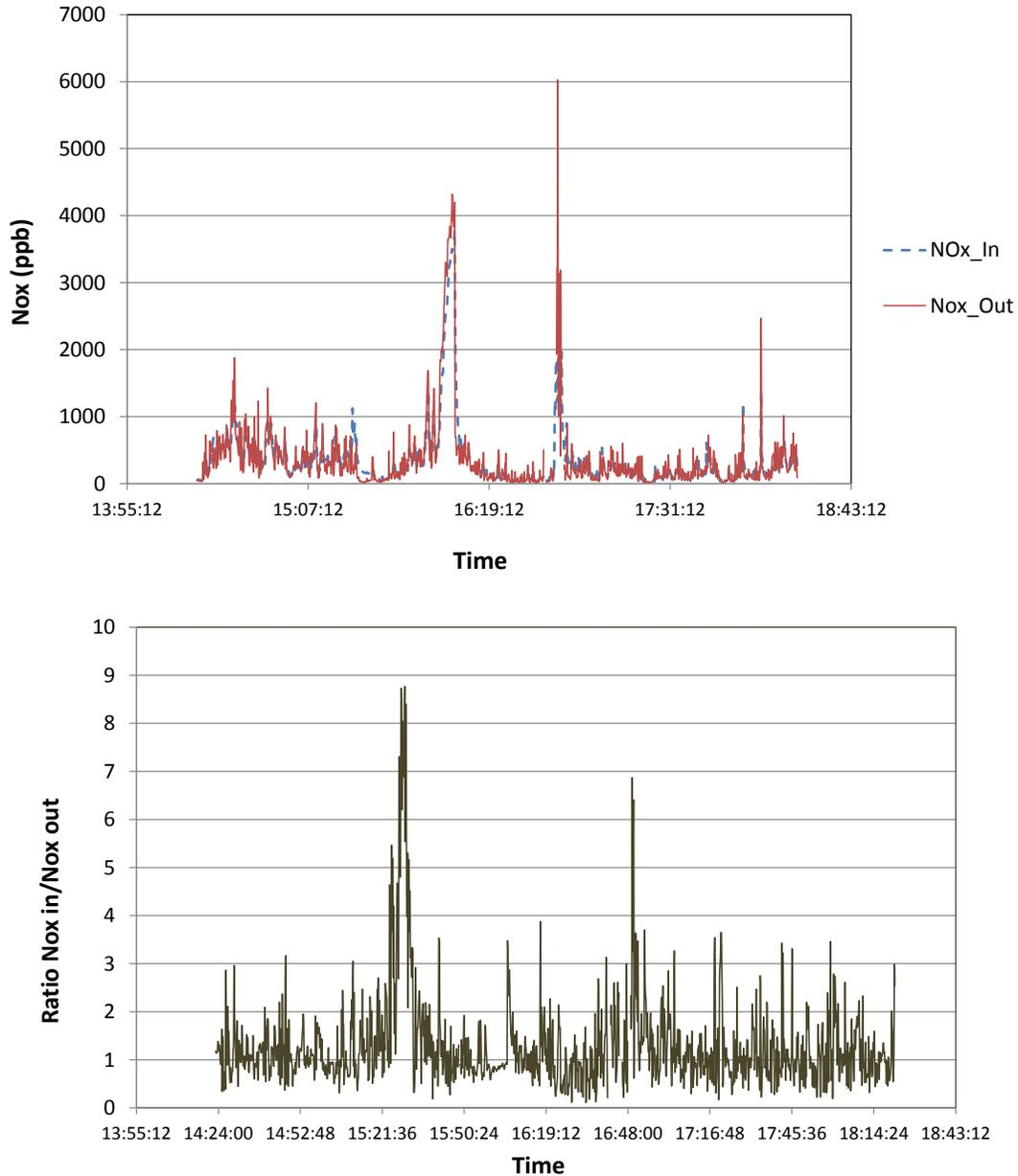
FIGURE 2. Time evolution of NO<sub>x</sub> concentrations inside and outside the vehicle cabin (top) and I/O concentrations ratio (bottom)
