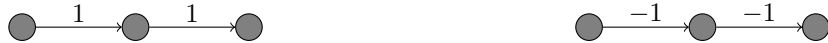
Figure 5: Counter-example showing that the conclusion of Theorem 3.1 does not hold when the parameters have opposite signs. If the hidden neurons are ReLU neurons, the left network implements R_\theta(x) = \text{ReLU}(x) (with \theta = (1 \ 1)^T ) and the right network implements R_{\theta'}(x) = -\text{ReLU}(-x) (with \theta' = (-1 \ -1)^T ). Equation (4) does not hold since there is a single path and the product of the weights along this path is equal to one in both cases, so that \Phi(\theta) = \Phi(\theta') = 1 (cf Section 2) while these two functions are nonzero and have disjoint supports.
