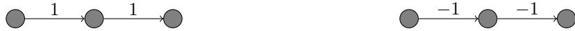
Figure 5: Counter-example showing that the conclusion of Theorem 3.1 does not hold when the parameters have opposite signs. If the hidden neurons are ReLU neurons, the left network implements R_\theta(x) = \text{ReLU}(x) (with \theta = (1 \ 1)^T ) and the right network implements R_{\theta'}(x) = -\text{ReLU}(-x) (with \theta' = (-1 \ -1)^T ). Equation (4) does not hold since there is a single path and the product of the weights along this path is equal to one in both cases, so that \Phi(\theta) = \Phi(\theta') = 1 (cf Section 2) while these two functions are nonzero and have disjoint supports.
