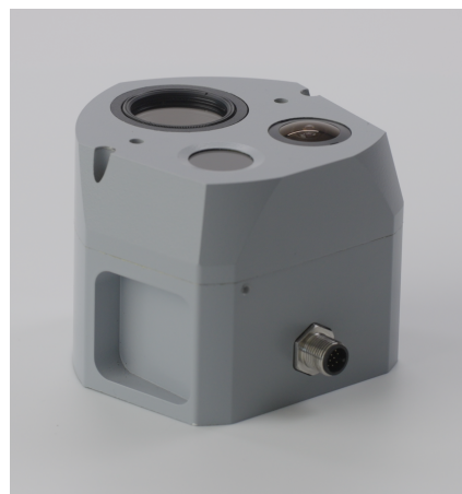
Figure 10. The SkyPASS Gen3-N sensor (size: 10.4 \times 9.9 \times 8.1 cm, mass: 567 g, max measurement frequency: 1 Hz) employs separate optical channels to image the sun, stars, and sky polarization to provide a highly accurate heading better than 0.1^\circ . Tracking sky polarization improves availability of the sensor in twilight, cloudy skies, and urban environments. Courtesy from Polaris Sensor Technologies Inc. (Huntsville, AL, USA), see https://www.polarissensor.com/skypass/ (accessed on 17 May 2024) for details.
