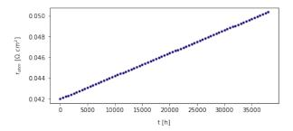
Figure 8: Temporal evolution of  $r_{ohm}$  at  $1A/cm^2$ .
