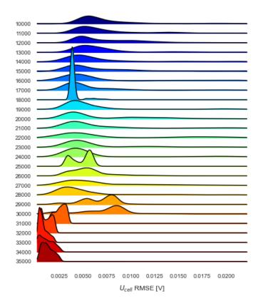
Figure 17: Distribution of the root mean square error of the voltage for different learning durations.
