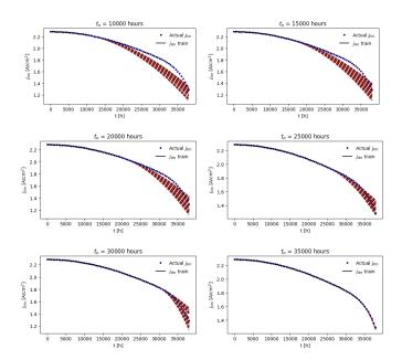
Figure 13: Simulation of  $500~j_{lim}$  curves for different learning durations. The red curves represent the simuled scenarios.
