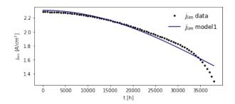
Figure 9: Fitted curves of  $j_{lim}$  with model1 (Equation 10).
