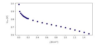
Figure 1: Initial experimental polarization curve.
