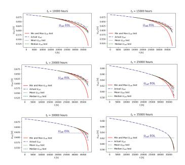
Figure 15: Statistics on the distribution of the voltage prediction by EKF for different learning duration.
