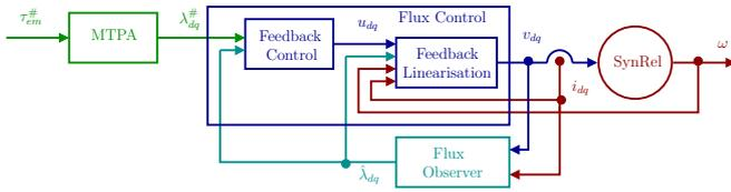
Fig. 4 Representation of the overall observer based flux controller.
