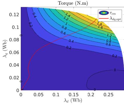
Fig. 3 Torque-flux characteristic and MTPA trajectory (red).
