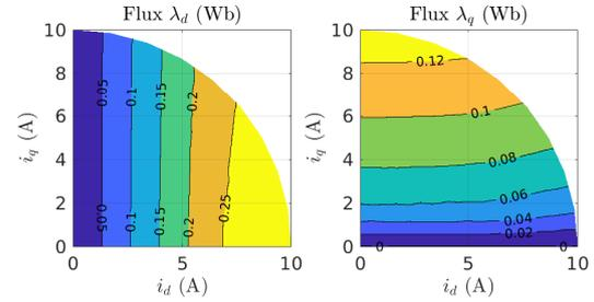
Fig. 2 Nonlinear flux-current characteristic obtained from FEMM.
