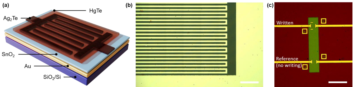
Figure S 6 Geometrical device from Figure 5. a. Schematic of the planar p-n junction. b. Optical microscopy image of the Ag_2Te pattern deposited onto SnO_2 layer deposited on gold layer. c. Optical microscopy image for the nanocrystal film coupled to a PZT ferroelectric layer (in green), whereas the red background correspond to SiN . Scale bars in the optical images correspond to 100 \mu m .
