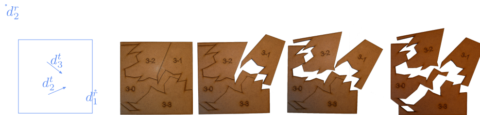
Figure 29: An assembly made of 3+1 parts: P_1 obeys a rotation around \mathbf{d}_1^r ; P_2 obeys both a translation along \mathbf{d}_2^t and a rotation around \mathbf{d}_2^r ; P_3 obeys a translation along \mathbf{d}_3^t
