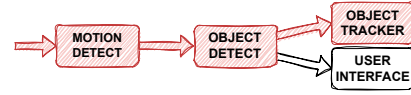
Fig. 1: DAG of the application, inspired from the surveillance camera use-case of [13]. The critical path is in red (used to measure end-to-end request latency).
