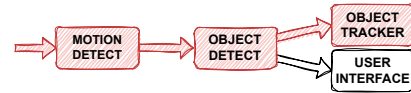
Fig. 1: DAG of the application, inspired from the surveillance camera use-case of [13]. The critical path is in red (used to measure end-to-end request latency).
