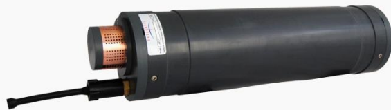
SeaFET pH autonomous logger (Acquired in 2015)
