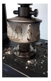
Figure 7. Presence of vertical cracks.
