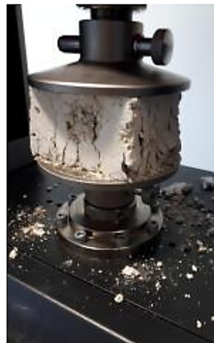
Figure 7. Presence of vertical cracks.
