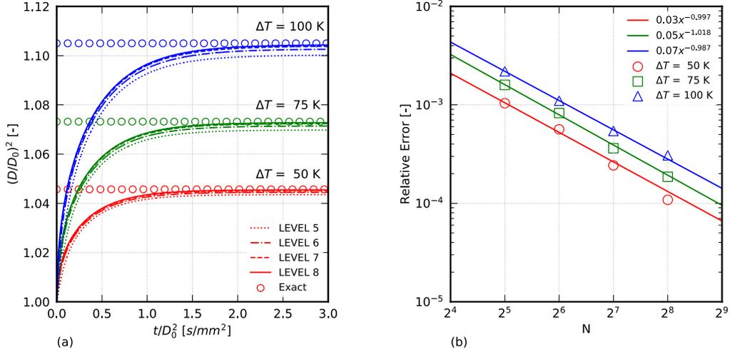
Figure 6: Evolution of the normalized square diameter for the droplet expansion problem at different  $\Delta T$  between the droplet and the environment (a); convergence rate for the droplet expansion problem (b) (<http://basilisk.fr/sandbox/ecipriano/run/expansion.c>).
