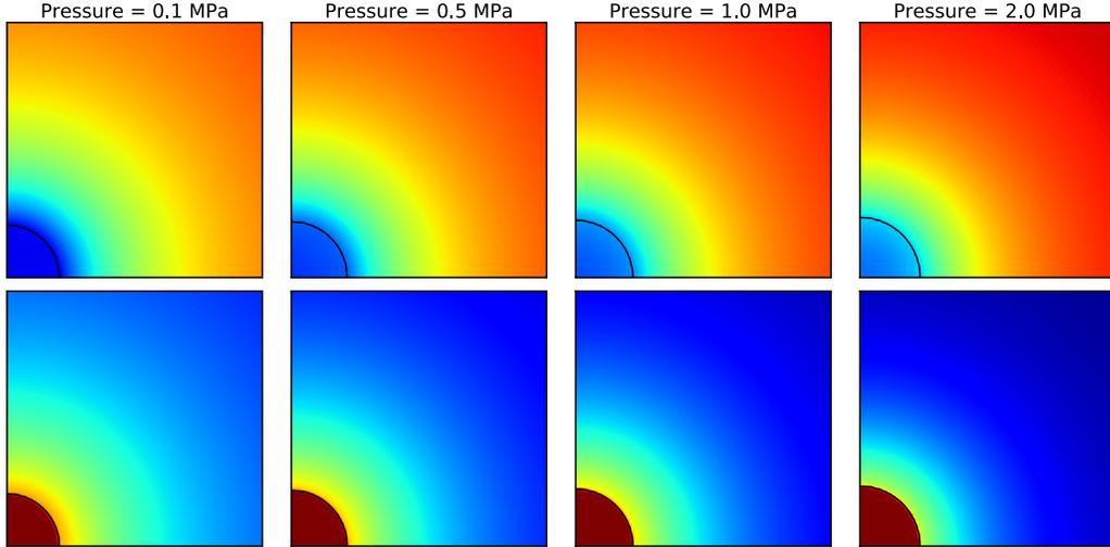
Figure 7: Maps of temperature (top) and n-heptane mass fraction (bottom) at different ambient pressures in microgravity conditions at  $T \approx 750$  K and time 0.6 s (<http://basilisk.fr/sandbox/ecipriano/run/microgravity.c>).
