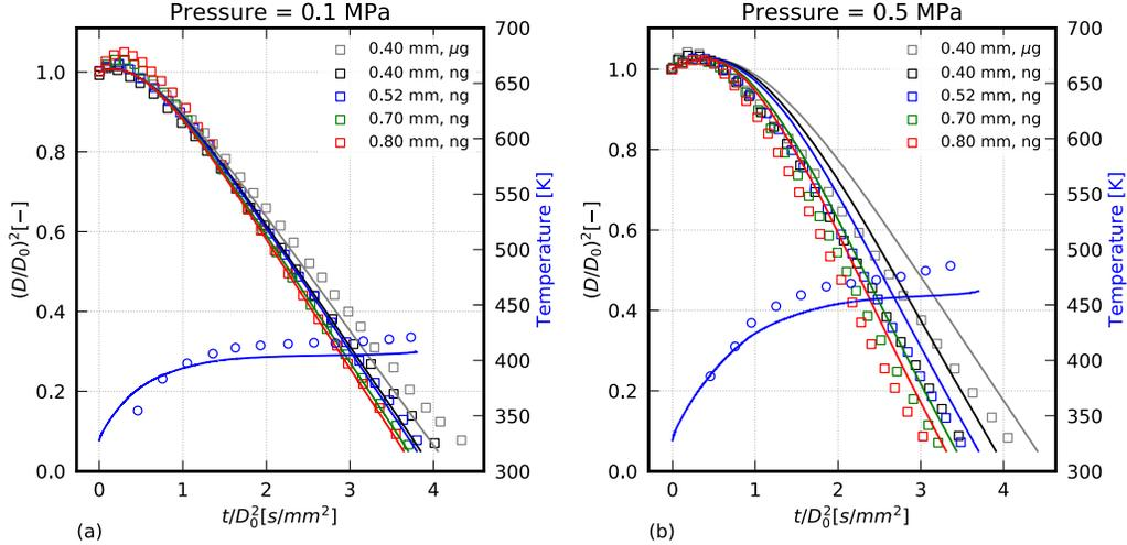
Figure 11: Normalized squared diameter and temperature profile for the n-decane evaporation in normal gravity conditions (ng) and in microgravity ( $\mu g$ ). Comparison with experiments by Murakami et al. [5] (<http://basilisk.fr/sandbox/ecipriano/run/normalgravity.c>).
