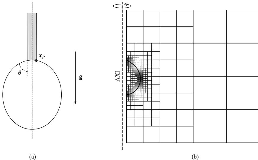
Figure 1: Simulation setup for suspended droplets in normal gravity conditions. Schematic representation of the droplet suspended on a solid fiber, with contact angle  $\theta$ , pinning point  $\mathbf{x}_p$ , and gravity  $\mathbf{g}$  (a); simulation setup for the axial-symmetric suspended droplet configuration, using an adaptive grid (b).
