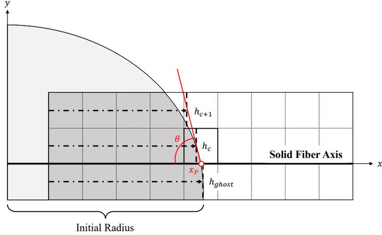
Figure 2: Schematic representation of the height function boundary conditions, where the black line represents the solid fiber surface, the white point is the pinning point  $\mathbf{x}_p$ , while  $\theta$  is the contact angle.
