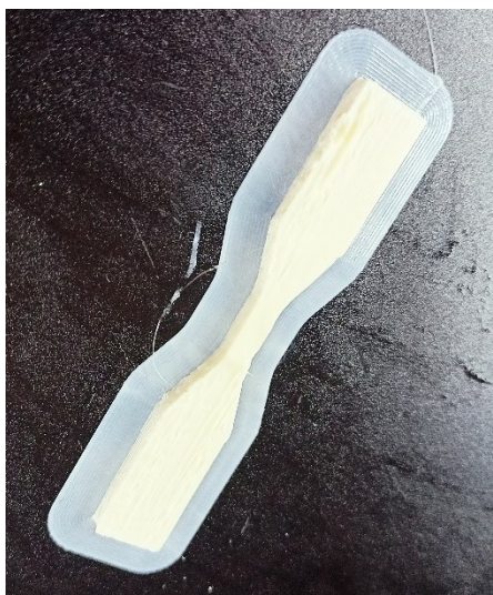
Figure S14 Printing of complex shapes of Extru_100 formulation: A) interior of cube pattern, B) Cube, C) Unidirectional printed tensile specimen, D) Gyroid structure.
