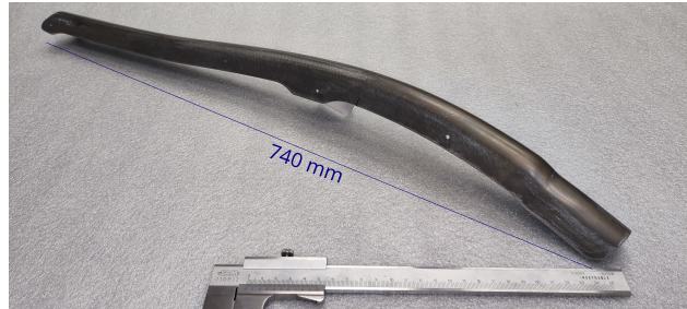
Figure 1. Aeronautical component of the A320 neo pylon after forming and contour machining.
