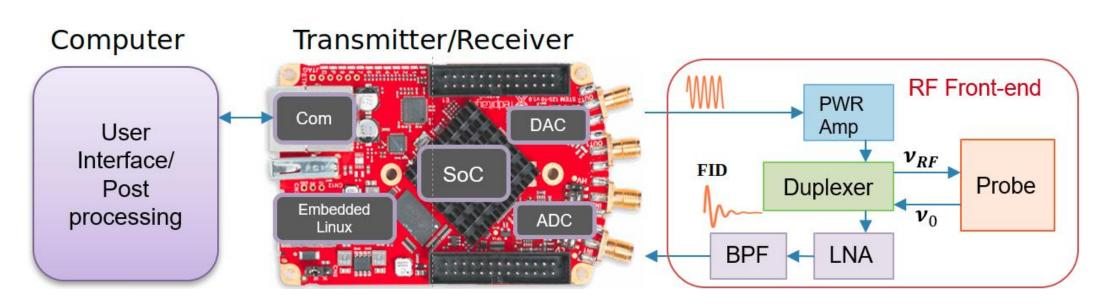
Fig. 2 New NQR spectrometer.
