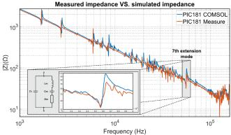
**Fig. 18.** Van Dyke circuit model of the setup in Fig. 17 around the 7<sup>th</sup> extension mode.
