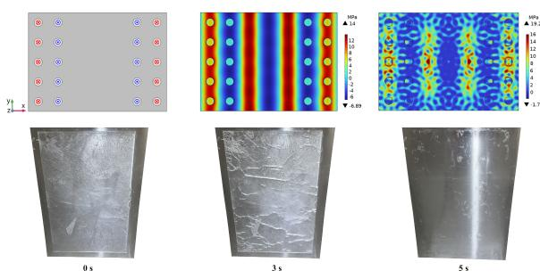
Fig. 17. Computation result of the 7th extension mode and its corresponding experimentation results.
