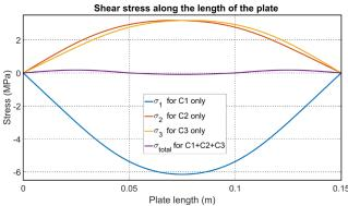
**Fig. 10.** Shear stress level traced along a line that runs the length of the plate at the 1<sup>st</sup> extension mode for one actuator at a time, and then all three together.
