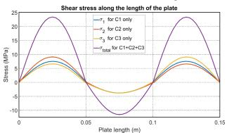
**Fig. 11.** Shear stress level traced along a line that runs the length of the plate at the 3<sup>rd</sup> extension mode for one actuator at a time, and then all three together.
