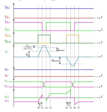
Fig. 21. ARCPI theoretical waveforms.
