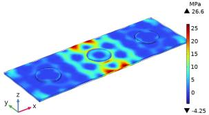
**Fig. 13.** Shear stress level at the 3<sup>rd</sup> extension mode around 59 kHz with free displacement on the x, y and z axis.
