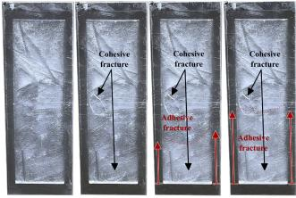
**Fig. 15.** Cohesive fractures and propagation of adhesive fracture at the 3<sup>rd</sup> extension mode.
