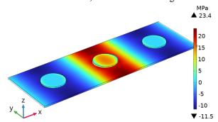
**Fig. 12.** Shear stress level at the 3<sup>rd</sup> extension mode at 59 kHz with zero displacement imposed on the y and z axis.
