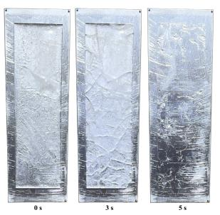
**Fig. 16.** Experimental result of deicing a 2 mm glaze ice layer at the 3<sup>rd</sup> extension mode of the rectangular plate.
