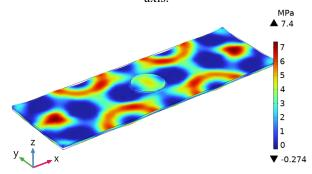
**Fig. 6.** Stress levels at the 1<sup>st</sup> extension mode around 20 kHz with free displacement on the x, y and z axis.
