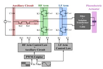
Fig. 20. Circuit topology of the ARCP Inverter.
