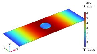
**Fig. 5.** Shear stress levels at the 1<sup>st</sup> extension mode at 20 kHz with zero displacements imposed on the y and z axis.
