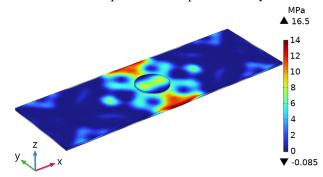
**Fig. 8.** Shear stress levels at the 3<sup>rd</sup> extension mode at 59 kHz with free displacement on the x, y and z axis.
