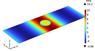
**Fig. 7.** Shear stress levels at the 3<sup>rd</sup> extension mode at 59 kHz with zero displacements imposed on the y and z axis.
