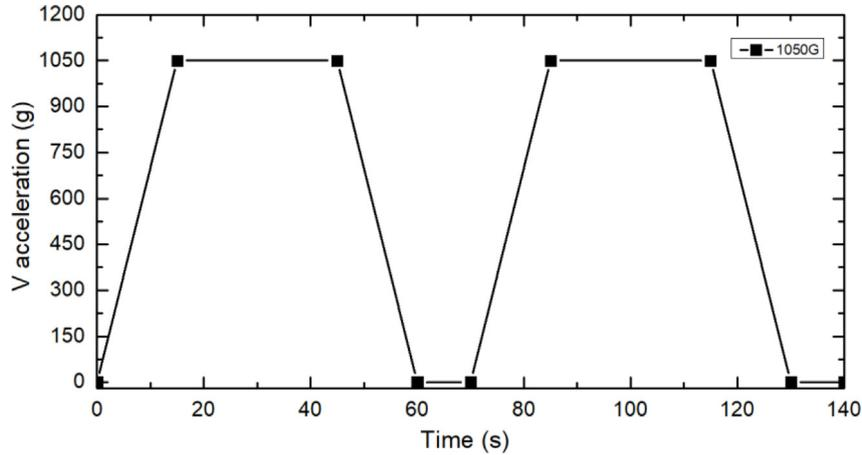
Fig. 4. SpinTest acceleration profile at 1050 g.
