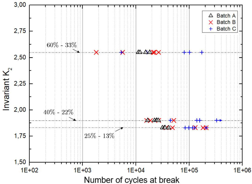
**Fig. 18.** S-N plots for different rubber batches.
