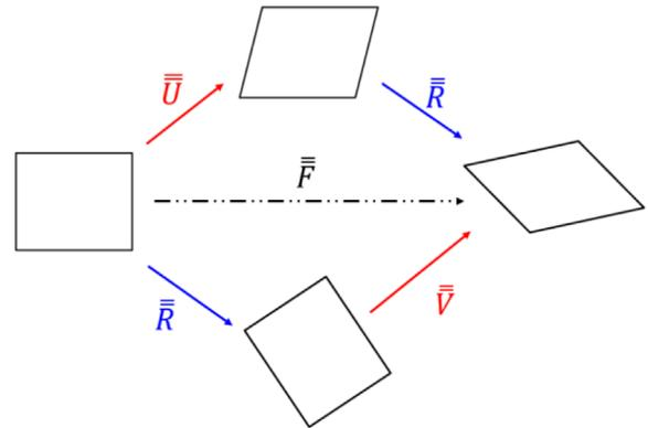
Fig. 11. Polar decomposition of the deformation gradient  $F$ .
