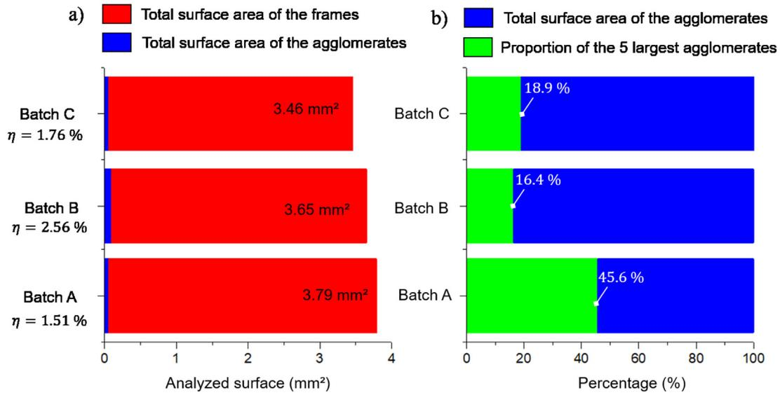
**Fig. 23.** (a) Demonstration of the surface area proportion of the agglomerates in the entire set of samples; (b) contribution of the five largest agglomerates. The percentage  $\eta$  corresponds to the surface area percentage of the agglomerates compared to the frames.
