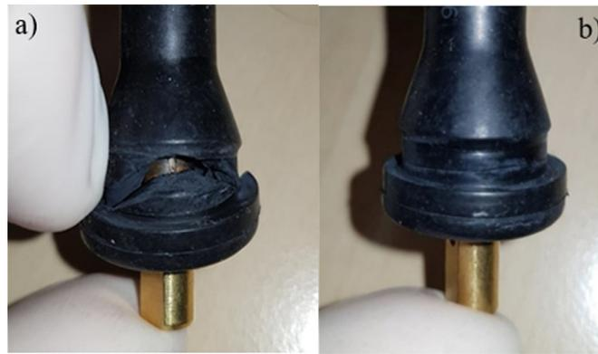
Fig. 2. Defective and operational valves after fatigue characterization.
