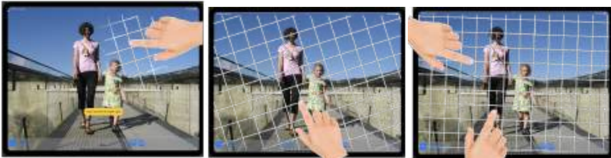
Figure 2: (a) Touching the screen to create a grid; (b) One-finger dragging to translate; (c) Two-finger dragging to rotate and dilate
