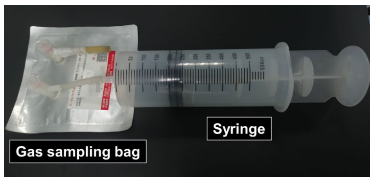
Figure S9. Volume measurement using a graduated syringe.
