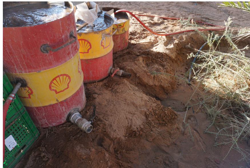
Flotation station realised by a scrap metal merchant from empty petrol tanks Tip: Use soft flexible hosepipe (garden hoses) of about 15-20 m.
