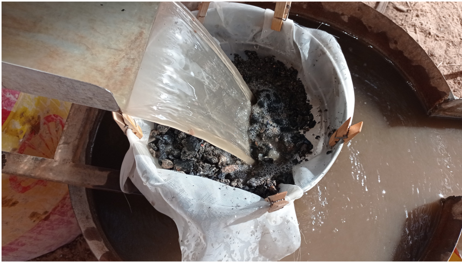
Calibrated flexible laboratory sieve (mesh 0.3 mm) fixed with clothes pegs on a rigid sieve and placed on a rack.
