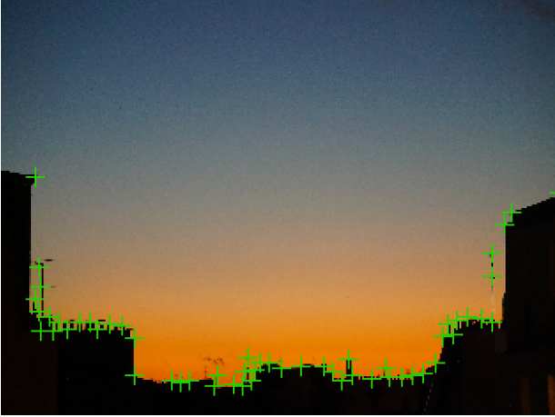
Figure 2. Example of keypoint analysis as performed by the OpenCV computer vision package. Each green cross is one salient feature or keypoint found.
