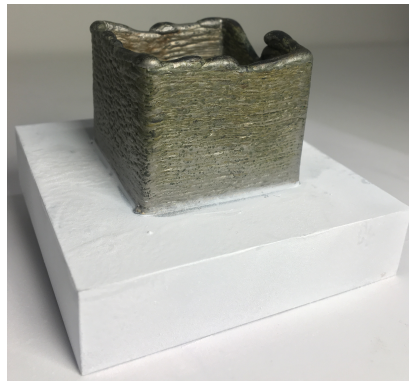
Fig 2 Part produced by wire-laser additive manufacturing.
