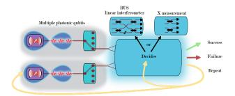
Figure 10: Hybrid RUS gate including spin qubits capable of emitting multiple entangled photons, an adaptive interferometer and detectors. The linear-optical interferometer is adaptive and depends on previous measurement outcomes. Horizontal black rectangles correspond to 50:50 beamsplitter, the inclined parallelogram corresponds to a  $-\pi/2$  phase shifter, numbered semiovals are photon-number-resolving detectors.
