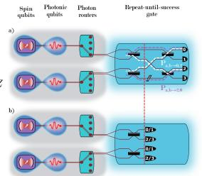
Figure 8: (a) Linear-optical interferometer with input spin quantum emitters. The paths  $P_{a,b\to0,2}$  and  $P_{a,b\to2,0}$  are represented in white and violet dashed lines respectively. The vertical red dashed line corresponds to the zone before the mode swap mentioned in the main text. (b) "Equivalent" linear-optical interferometer for distinguishable photons.
