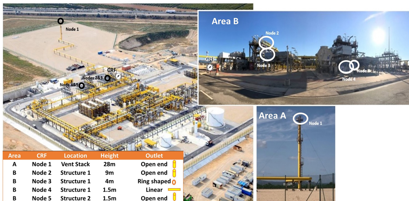
Figure 1. Aerial view of the Enagas site in Spain and node locations (white circles). The controlled-release facility is indicated by a white disk marked “CRF”.
