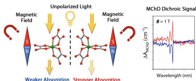
Figure: Principle of MChD in a chiral magnetized system (left) and typical MChD spectra (right).
