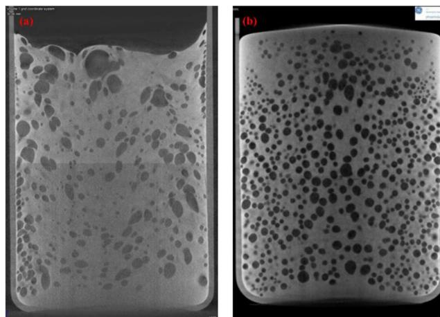
**Fig. 6.** Effect of dose rate on the shape, size and number of bubbles created, (a) BWPs at 5000 Gy/h and (b) BWPs at 400 Gy/h tomography extract from Mouazen's thesis [29].
