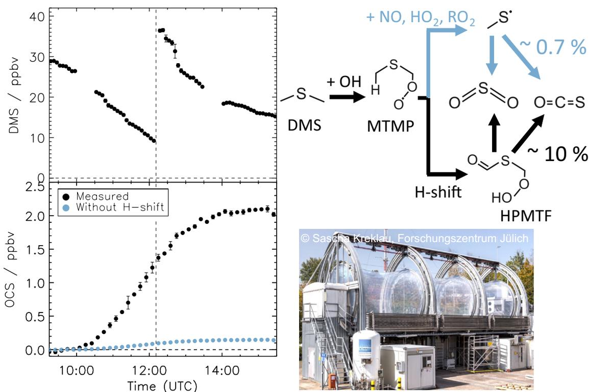
**FIG. 5.** Evidence for higher-than-expected formation of OCS in the OH oxidation of DMS due to H-shift reactions following the HPMTF formation path (Veres et al. 2020) in experiments carried out in the SAPHIR atmospheric simulation chamber.
