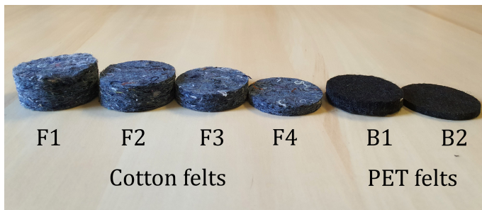
Figure 1: Felt samples thermobonded at different thicknesses (sample diameter, 45mm).
