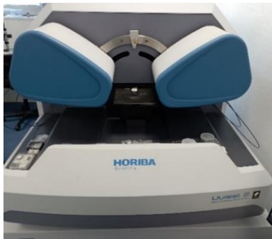
Fig. 10. Horiba Uvisel 2 spectrometer used for the ellipsometric measurements.
