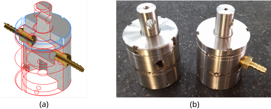
Figure 4: (a) CAD project of the coupling/cooling parts for the actuators and (b) the final parts in stainless steel. See “cooling of actuators” in Figure 2 for visualizing these parts in the setup.
