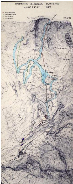
Figure 4: Preliminary design of Pic d'Artsinol ski lifts, 1979
