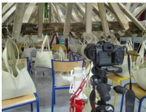
Figure 12: technique to measure the deflection
