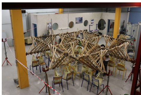
Figure 11: Loading of the truss
