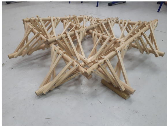
Figure 8: View of the model with hypar upper and lower layer
