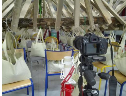
Figure 12: technique to measure the deflection
