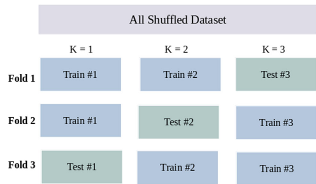
Fig. 8 Example of K-Fold cross validation method
