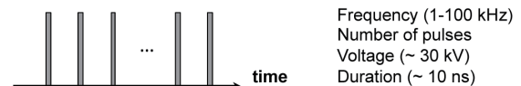
Fig. 1 Schematics of the time chart of (a) conventional spark and (b) NRP, and those adjustable parameters.
