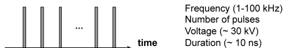
Fig. 1 Schematics of the time chart of (a) conventional spark and (b) NRP, and those adjustable parameters.
