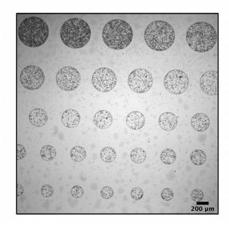
FIG. 1. Experimental setup. (a) Schematic drawing of a PDMS chip with shallow cylindrical wells of varying diameters. The algal solution is deposited in the wells, which are then sealed with a glass slide. The chip is exposed to blue light from the side. (b) Bright-field microscopy image of an array of 23 cylindrical wells of different diameters and identical algae concentrations. Cell bodies are visible as black dots inside the wells.
