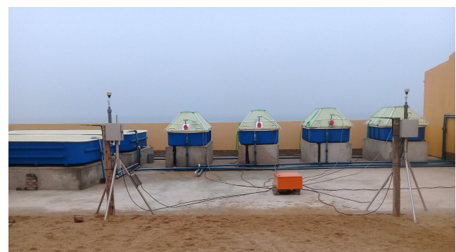
Figure 2: E-samplers (mounted on tripod stands) that were used to concurrently measure \text{PM}_{2.5} (left) and \text{PM}_{10} (right).
