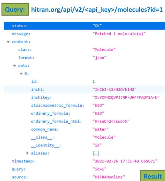
Fig. 40. Sample JSON response for the REST API query requesting molecule information, with an additional restriction imposed on the HITRAN ID value. The JSON fields contain the information on the molecule entry with the id=1 (water vapor).
