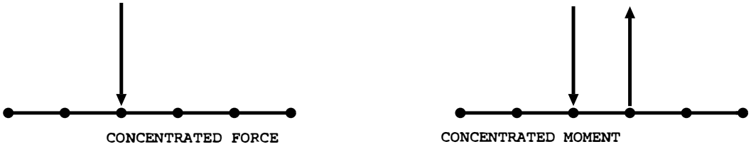
Figure 1 Concentrated forces and moments
