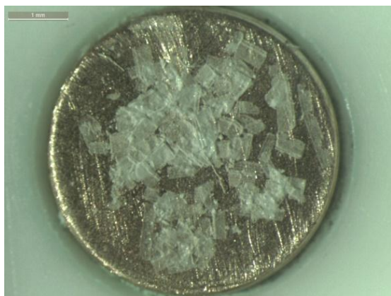
Figure S9. Photo obtained by stereomicroscope of the slices of resin incorporating [\text{Gd}_2(\text{L}^*)_2(\text{ox})_2(\text{H}_2\text{O})_2] deposited on the surface of the fixed copper electrode of the ferroelectric device.
