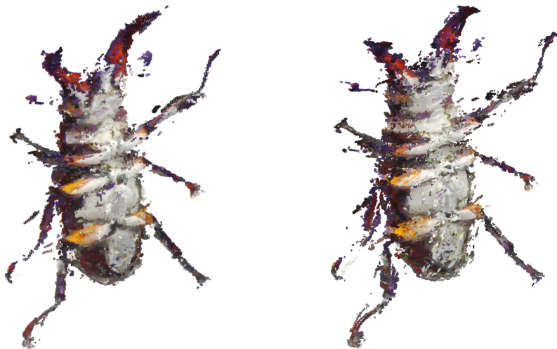
Figure 28 Comparison of our RMVS method, tested on the same 24 real images of the beetle (see Figure 24). We used either the IoR value estimated by the method illustrated in Figure 23 ( n_2 = 1.50 ), or a slightly overvalued IoR ( n'_2 = 1.56 ). The first result is obviously more accurate.
