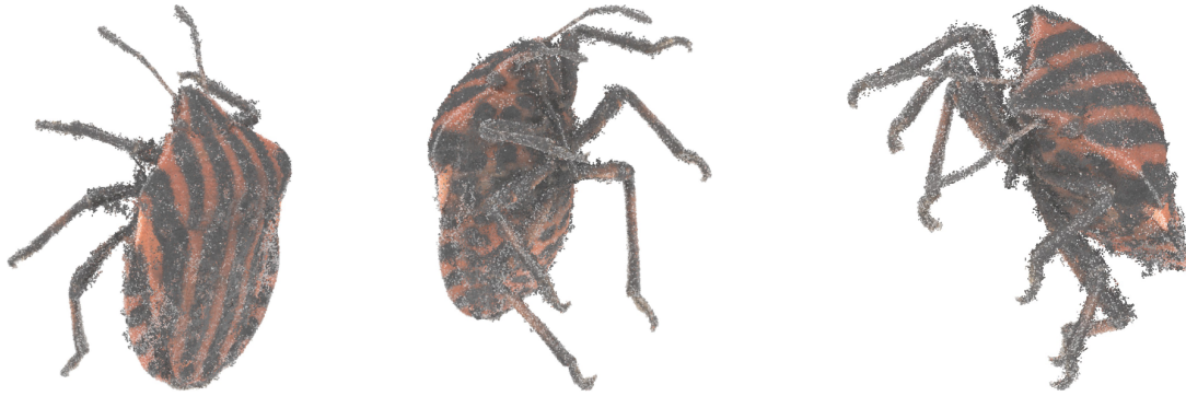
Figure 16 3D reconstruction of the graphosoma immersed in an epoxy resin regular dodecahedron, viewed from three angles. This was created using our RMVS solving method from 18 images such as those in Figure 15, followed by refinement using the Connected-component labelling tool of the Cloud Compare software.
