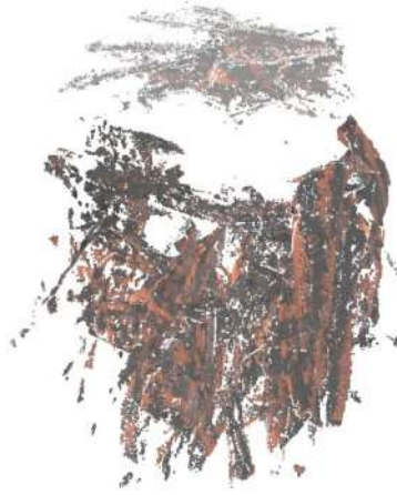
Figure 9. 3D reconstruction obtained by MVS, without taking refraction into account: because of the demultiplication of the image, the graphosoma is badly reconstructed, and it even appears copied three times.
