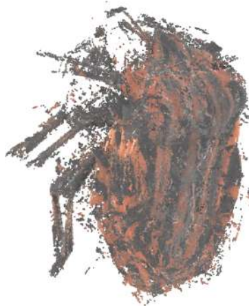
Figure 13. 3D reconstruction by MVS, from 18 images such as those in Figures 11-a and 11-b: due to the lack of consistency between the eight 3D point clouds, ghost legs and antennae appear.
