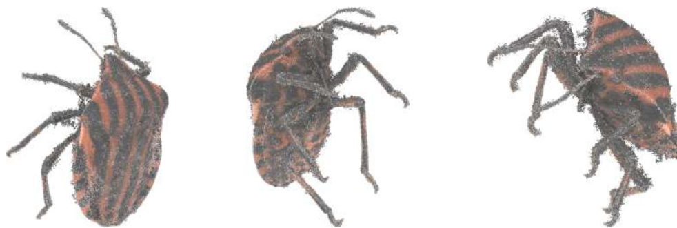
Figure 16. 3D reconstruction of the graphosoma immersed in a regular dodecahedron of epoxy resin, seen from three angles, obtained by our RMVS solving method from 18 images such as those in Figure 15, after cleaning with the Connected-component labeling tool of the Cloud Compare software.
