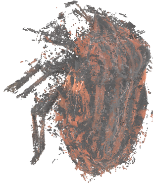
Figure 13 3D reconstruction using MVS from 18 images such as those in Figures 11-a and 11-b, results in ghostly legs and antennae due to inconsistencies among the eight 3D point clouds.
