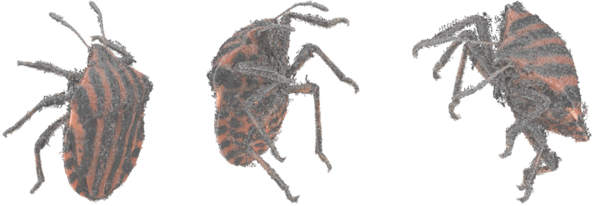
Figure 8 Result of Figure 7 after “cleaning” the 3D point cloud by the Connected-component labelling tool of the Cloud Compare software.
