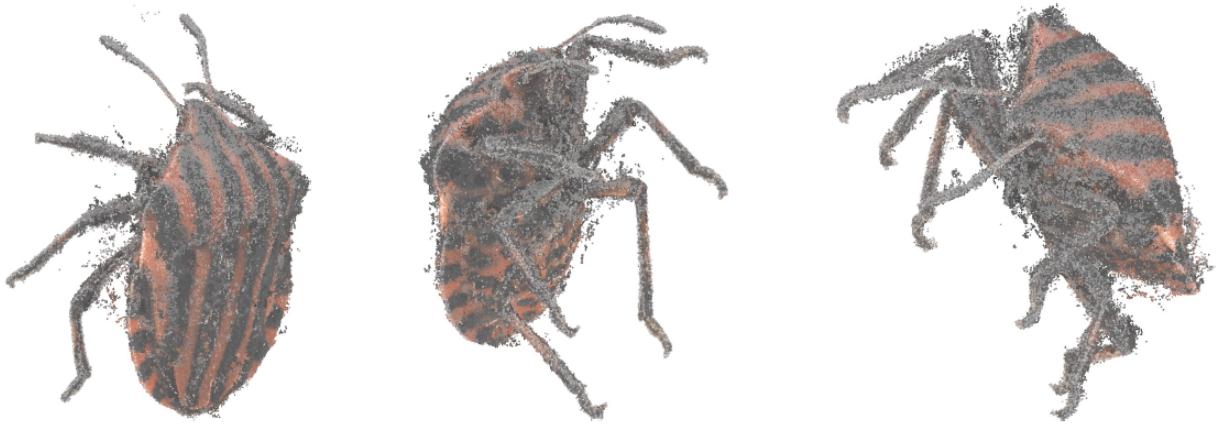
Figure 7 3D reconstruction of a graphosoma immersed in a cube of epoxy resin, seen from three angles, obtained by our RMVS solving method from 18 synthetic images such as those in Figure 6.
