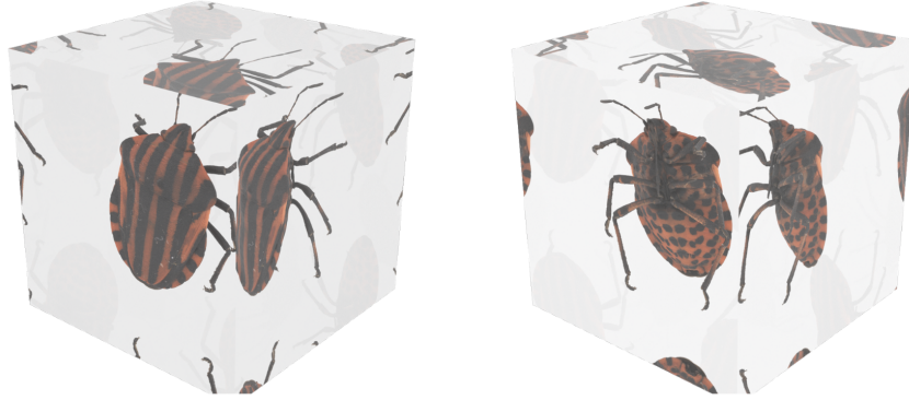
Figure 6 Two synthetic images (among 18) of a graphosoma immersed in a cube of epoxy resin. In both cases, the insect is visible through three faces of the cube (only partially, regarding the top face). Due to reflection phenomena, fragments of the object are visible at the borders of the immersion medium. These image fragments have not been used by our solving method. Source of the 3D model: Digital Archive of Natural History 55 .
