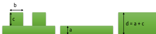
Fig. 9. Schematic of the periodic structure compared to two monolayers of thickness ( a ) and thickness ( a + c ).
