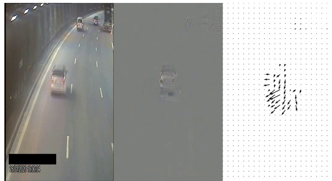
Fig. 1. Visualization of a video stream frame alongside its compressed representation. From left to right are the original RGB frame, the residual image and the Motion Vector (MV) representation. Only the moving vehicles generate information to be compressed. Note that motion vectors point in the opposite direction of the vehicles flow as they refer to previous frames.
