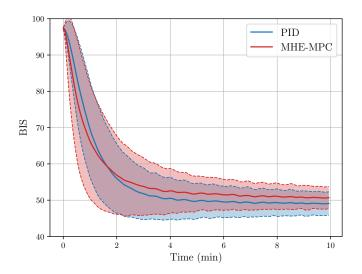
Fig. 3. Mean BIS over the 500 patients for the two controllers. The plot is the mean value  $\pm$  standard deviation.
