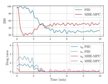
Fig. 4. BIS values for the worst case of each controller (in terms of undershoot) for the two controllers.
