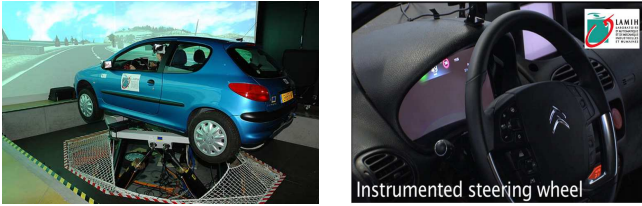
Fig. 4. SHERPA simulator (left) and its steering system (right).
